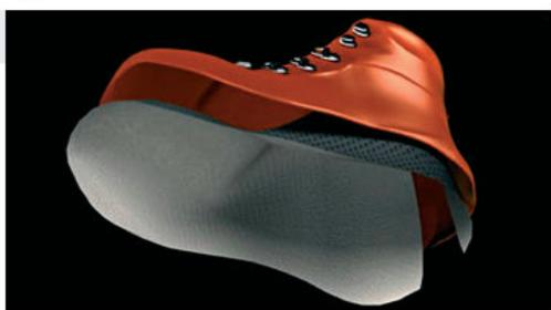
The OutDry® waterproof and breathable membrane is positioned inside the upper already stitched and closed, with lace hooks already placed;
