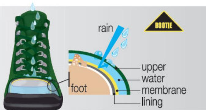
Conversely, with OutDry® technology the membrane is steadily bonded to the upper inner side and there is no space in between. Water remains therefore out of the shoe and the breathability is constantly maintained.
