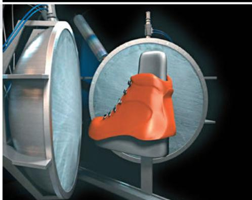
Lamination step is made by the patented diaphragm press (molding technology derived from aerospace industry) capable to laminate the membrane on 3D surfaces;
