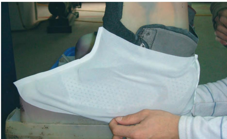
*Nextec OutDry membrane positioned on an upper*
