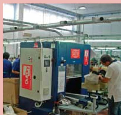
MEMBRANE SETS ARE BONDED IN THE PATENTED PRESS
